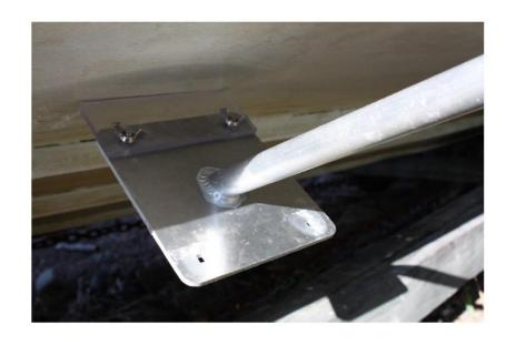
Cleaning scrape for the removal of barnacles and other biofouling organisms (Photo: Keep the Archipelago Tidy)
