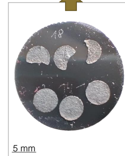
Sample holder with CCM for analysis
