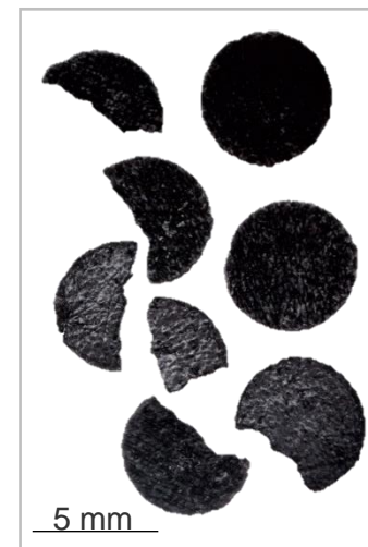
Delaminated and ruptured CCM + electrode powder
