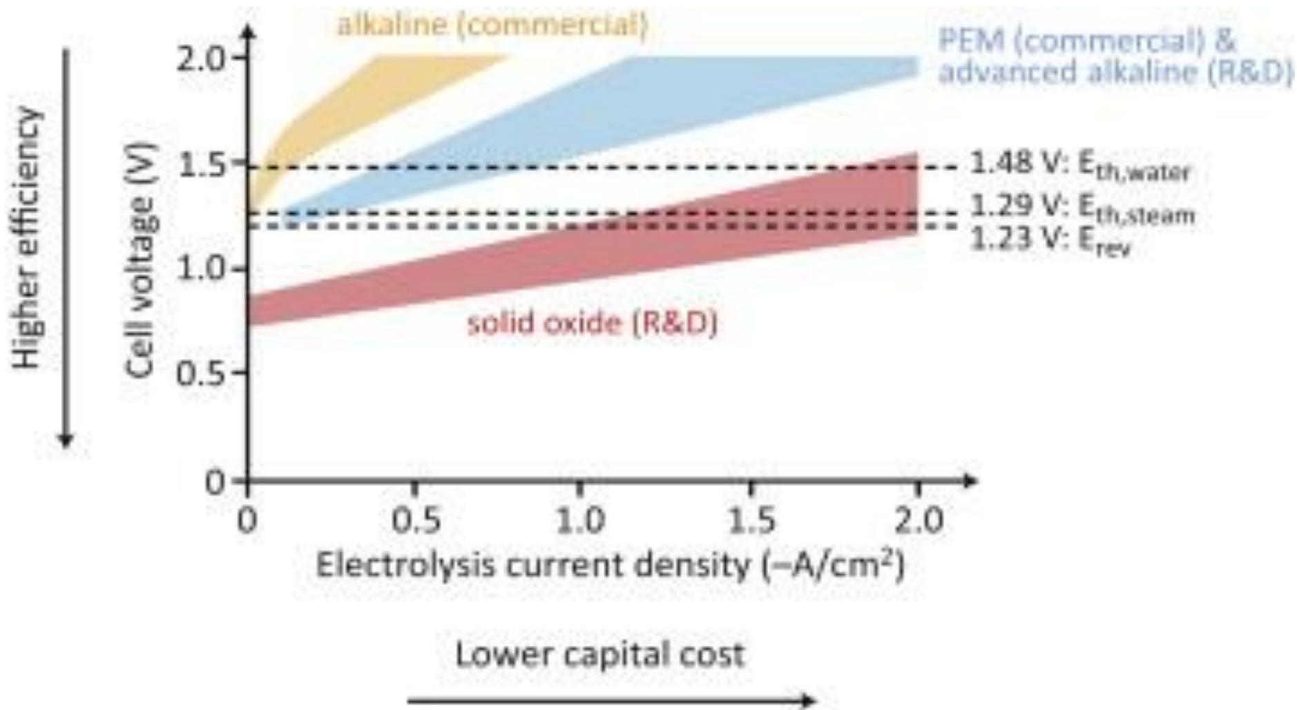
Typical ranges of polarization curves for different types of state-of-the-art water electrolysis cells.  $E_{th,water}$  and  $E_{th,steam}$  are the thermoneutral voltages for water and steam electrolysis, respectively.  $E_{rev}$  is the reversible potential for water electrolysis at standard state.
