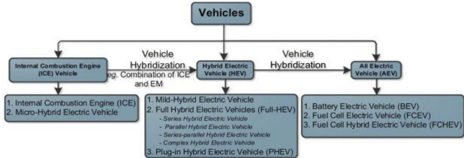
Fig. 4. Various classifications of a vehicle [2].
