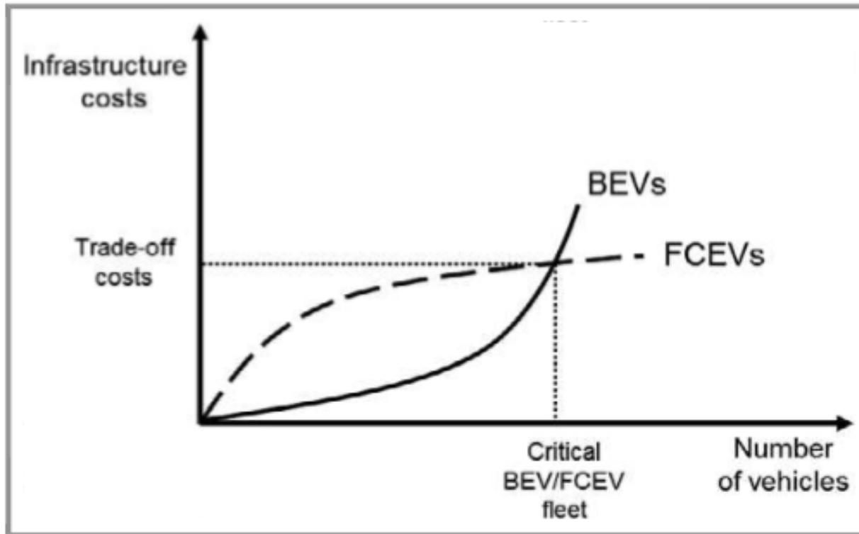
**Figure 2.** Qualitative investment needs for establishing a BEV recharging infrastructure vs a hydrogen refueling infrastructure for FCEVs.
