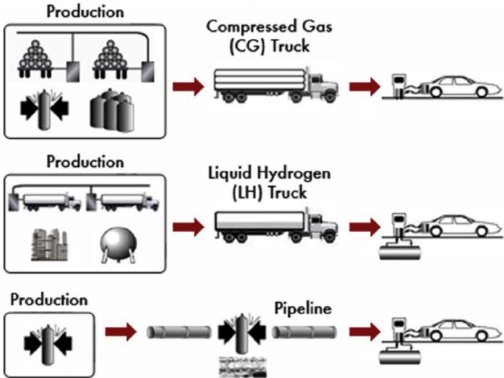
Fig. 4. Hydrogen delivery pathways. Source: [55].
