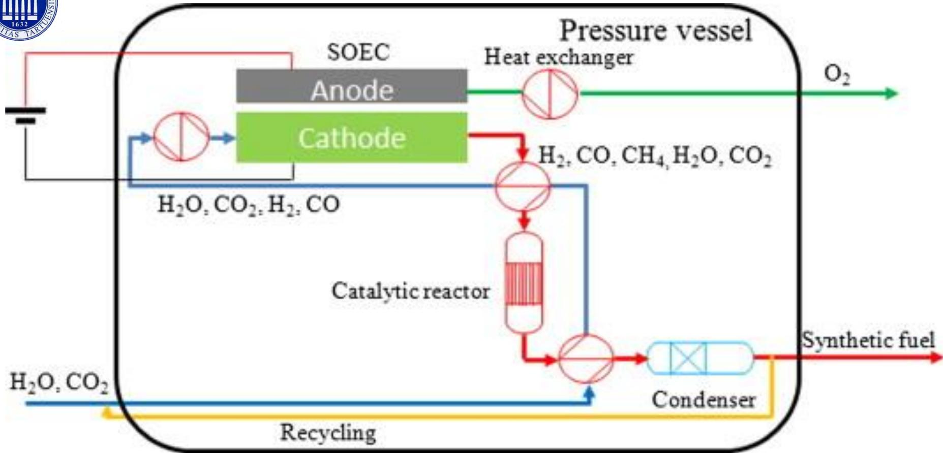
Sketch of a synthetic fuel production system based on a heat exchanger reactor coupled with high pressure co-electrolysis of  $H_2O$  and  $CO_2$ .
