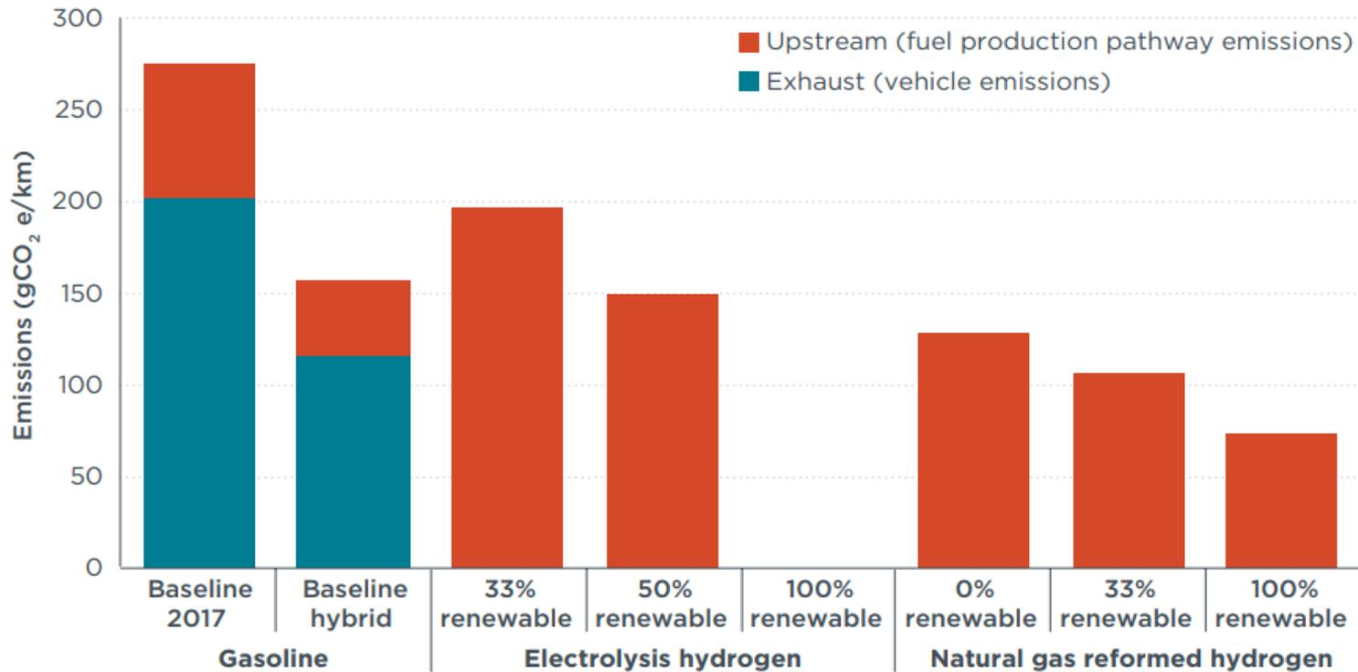
**Figure 3.** Hydrogen fuel cell vehicle CO<sub>2</sub>e versus conventional and hybrid gasoline vehicles.
